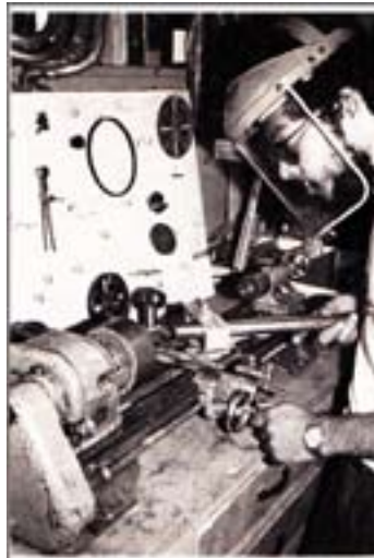
Angel Rodriguez mitres tube ends in his Seattle, Washington shop. The frame below, a track model built for partner Glenn Erickson, is made with graphite tubing. (Bicycle Paper photos)
